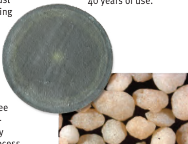
CT form of RONOZYME® ProAct and its results on a black filter paper in a dust measurement
