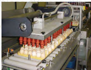
E-CAT In Ovo Eginject system transfer module: eggs are lifted from the setter tray (in yellow on the right side of the photo) and are then brought through a pendular movement in the hatcher basket (in white on the left).
