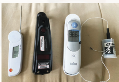
Fig. 1. Thermometers suitable for measuring embryonic or egg surface temperature.
