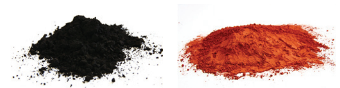
Two forms of copper oxide; left, Cupric oxide (CuO) copper(II) oxide, right, Cuprous oxide (Cu 2 O) Copper(I) oxide.
