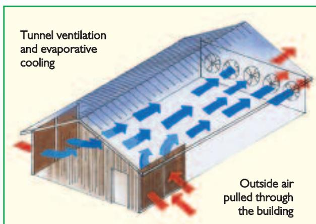
building interior. This dual process is known as evaporative cooling and tunnel ventilation, and it controls the interior temperature and quality of air.
