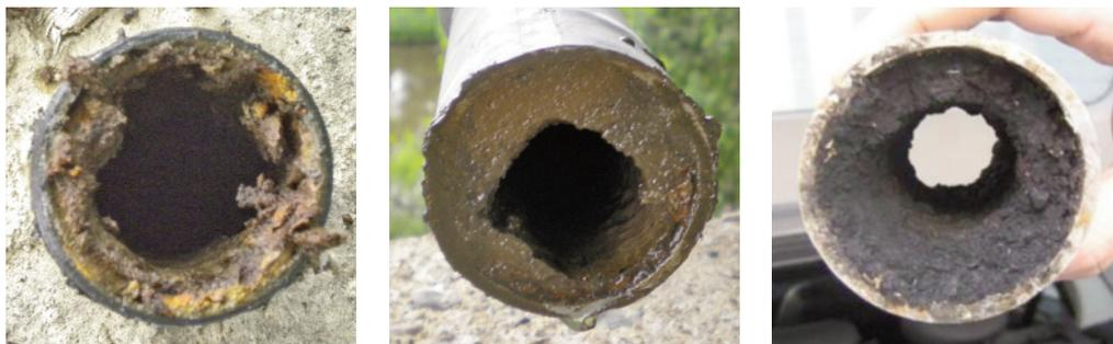
**Fig. 2. Transversal section of pipes and conduits with biofilm.**
