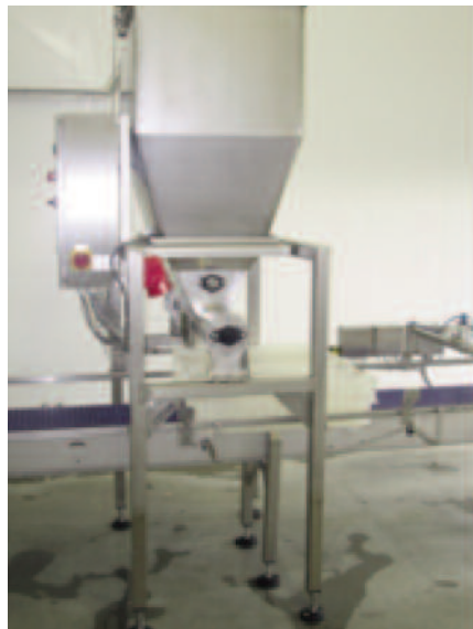
The unit for dispensing feed into the HatchBrood basket.
