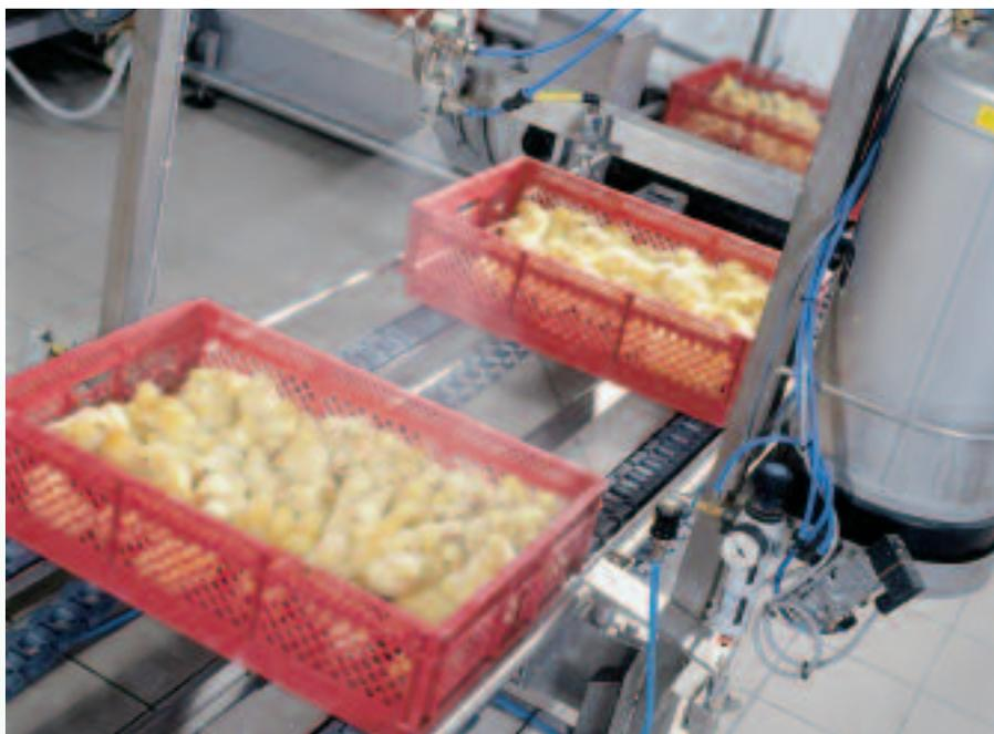
***In line spray administration of vaccine to day old chicks in the hatchery. It is important that spray equipment is correctly calibrated to administer a consistent droplet size. Too fine a spray may result in excessive post vaccination reactions.***
