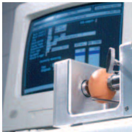
External quality. Eggshell breaking strength measurements being taken at Hendrix Poultry Breeders' test laboratory.
