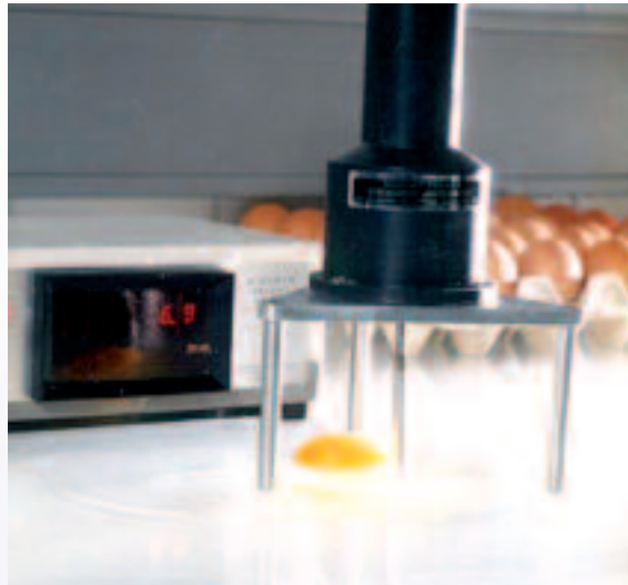
Internal quality. Haugh units are calculated by measuring the thickness of the egg white. Haugh units and internal egg quality are particularly important in the Japanese market where consumption of raw eggs is popular.
