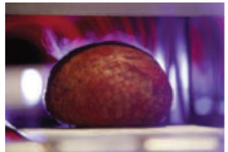
**In addition to achieving the smoking and some surface texturing, surface heat applied by the pasteuriser causes a Maillard reaction for the browning. So, after about a minute, instead of hours, the product can be retail packaged with no further post packaging pasteurisation required.**
