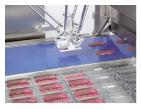
Weber's slicers, skinners and icers, the basic material is high grade stainless steel. The working space of the robot is enclosed by panes and doors made of transparent Macrolon.
