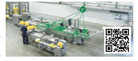
room, is ideally installed as a set. Meggsius Count is a camera system that counts the eggs just before the transfer to the central collection belt and works even in dark and dusty houses.
