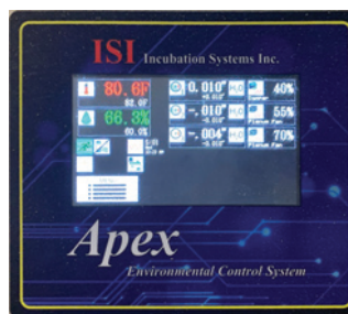
An example of a room controller featuring proportional control.
