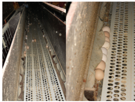
Eggs unable to roll on to the conveyor belt and a faecally contaminated nest box mat.
