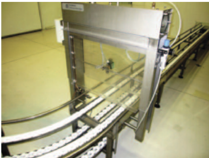
Left, the spray vaccination unit and, right, one of the mobile fans which circulates air in the chick holding area.
