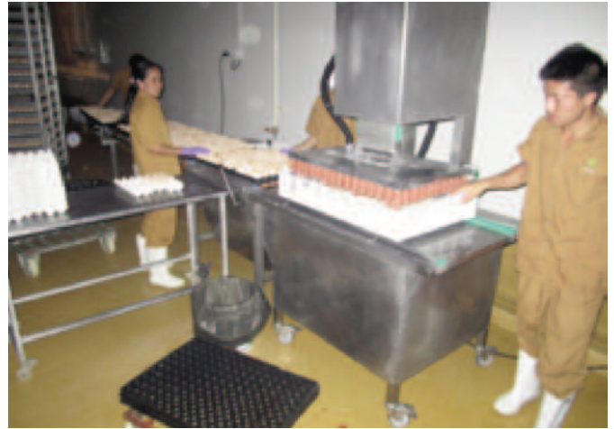
Left, eggs being fed into the transfer machine and, right, being placed in the hatcher basket.
