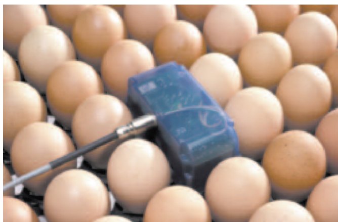
OvoScan installed on a setter tray.
