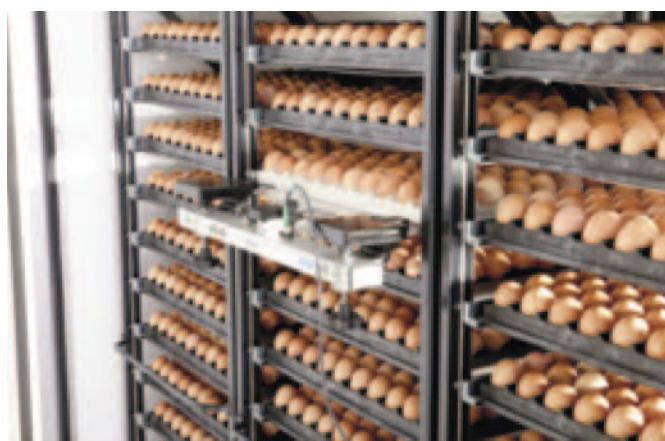
Dynamic Weight Loss System installed in a trolley.
