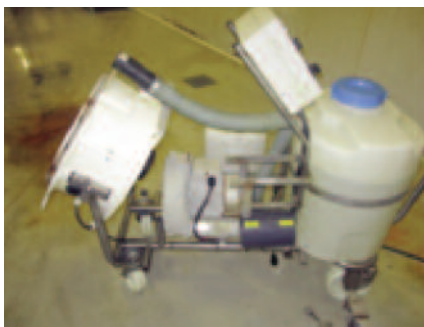
The equipment for generating an airborne mist of Nontox to disinfect rooms in the hatchery.
