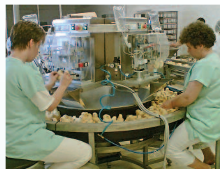
A four person Autovac injection carousel in operation, running up to 12,000 double injections and sprays per hour.
