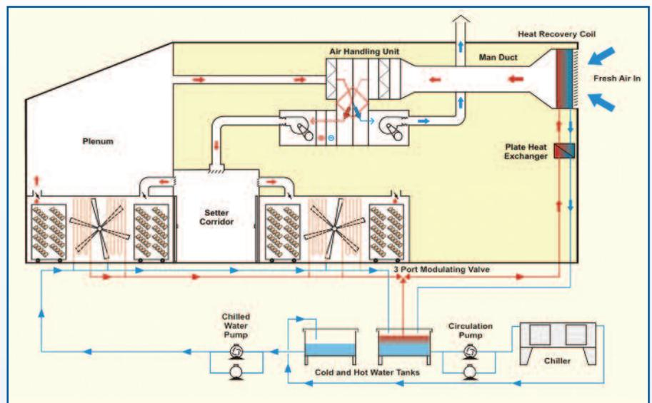
**Fig. 1. Diagram of the heat recovery and energy management system. Top right is the heat recovery coil through which warmed 'cooling' water from the setters is passed. Fresh incoming air passes over the warmed coil using recycled heat for the hatchery rooms. Heat exhausted from the setters is also used to further warm the incoming air in the air handling unit.**
