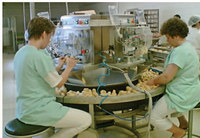
A four person Autovac injection carousel in operation, running up to 12,000 double injections and sprays per hour.
