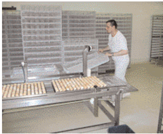
One person feeds empty hatcher baskets and full setter trays into the transfer machine.
