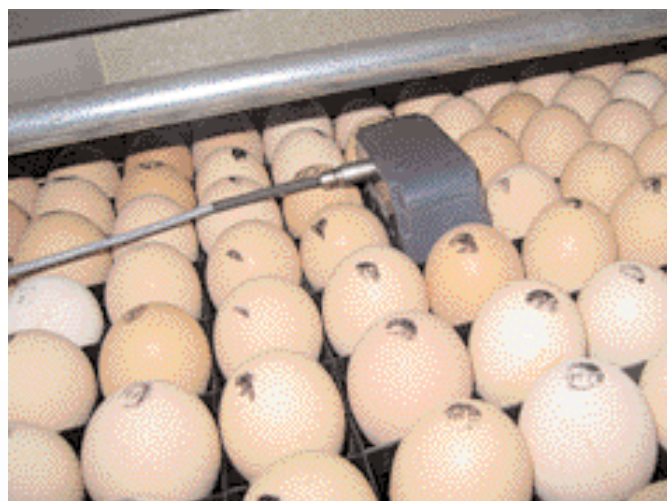
The Petersime specialist egg weighing system and their Ovoscan egg temperature monitoring system.
