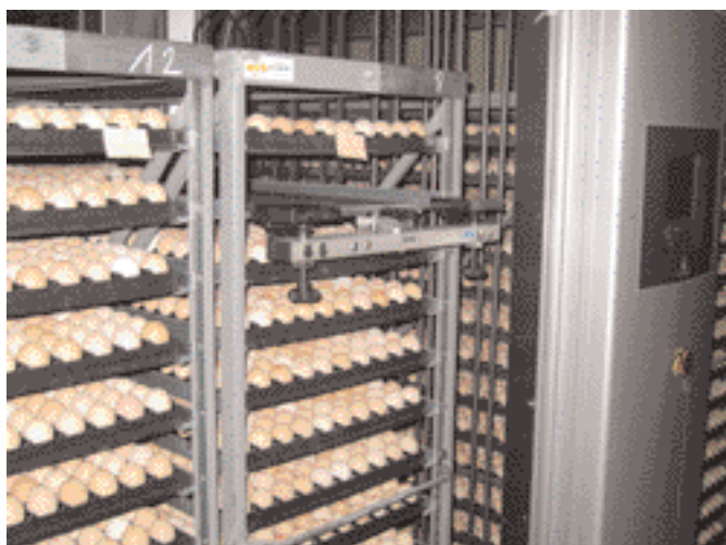
The Petersime specialist egg weighing system and their Ovoscan egg temperature monitoring system.
