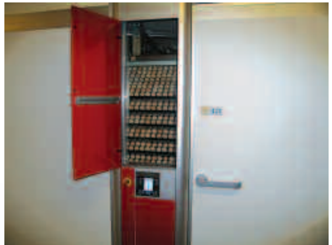
The new generation of Pas Reform setters with their new control panels and inspection window.
