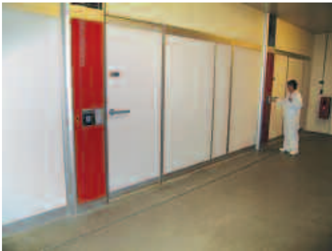
The new generation of Pas Reform setters with their new control panels and inspection window.
