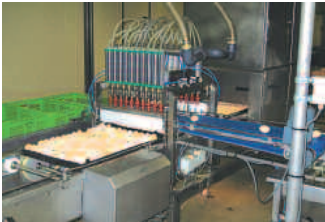
Egg transfer/candling using Viscon equipment and, below, the end result – quality chicks.
