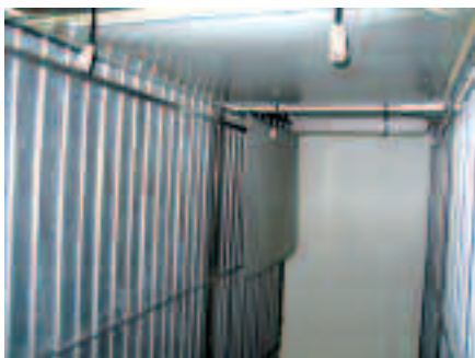
Left, inside the setters at cleaning. Special curtain flaps assist air flow and the cleaning process. Right, hatches ready for pulling.
