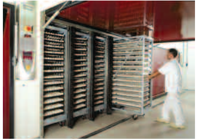
The original setters and, right, the new version with the up and over doors. Note how less space above the machine is required in the corridor.
