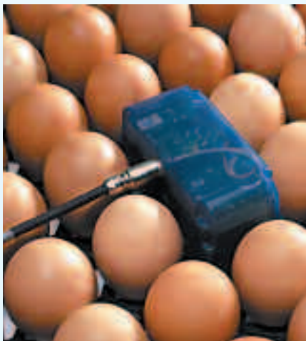
Petersime OvoScan egg shell scanner for bio-response controlled temperature. The Focus controller automatically adjusts the air temperature inside the incubator to achieve a preset level during all phases of incubation.
