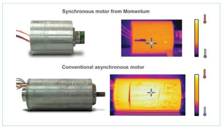
Temperature tests have shown that a 380 watt drum motor with IE2 efficiency rating gets around twice as hot as a synchronous drum motor with the same power rating and IE4 efficiency.
