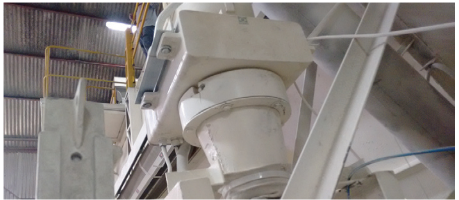
High access points on snack and bulk ingredient lines add to the health and safety risks when testing the performance of metal detectors.
