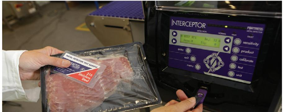
**Single pass product learning and automatic calibration stops operatives constantly resetting and recalibrating the metal detector for different pack sizes.**
