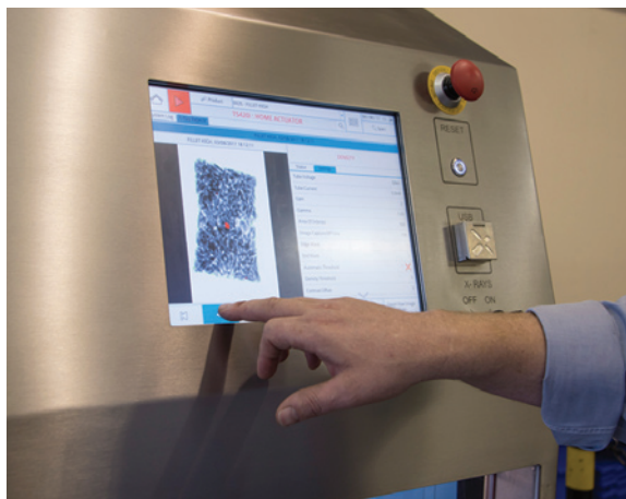
For food packaged in cans, tins or foil, x-ray inspection systems can play a critical role alongside metal detection.
