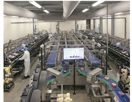
An automated picking system.
