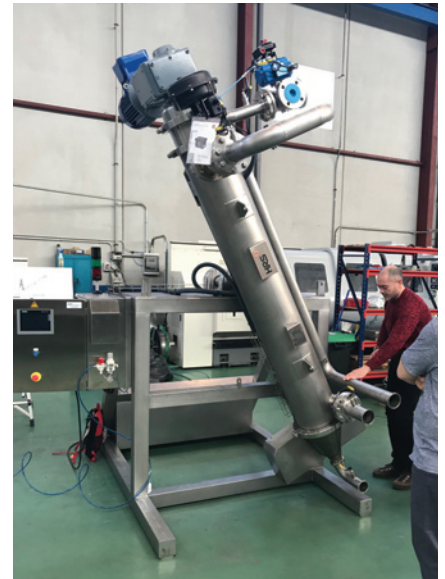
A skid-mounted version of the HRS R Series of scraped surface heat exchangers undergoing trials in the production of wax.
