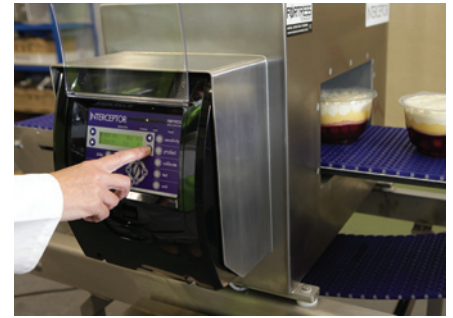
Using multi-frequency technology, Fortress developed and launched the new Interceptor range to help combat product and orientation effect.
