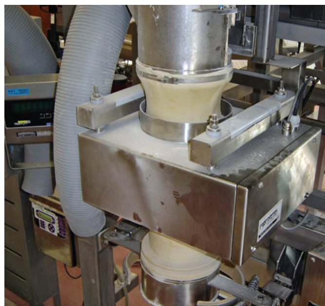
The Gravity Ultra+ metal detector now features a retractable reject unit for easier deep cleaning.
