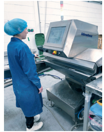
The Dylight X-ray inspection system by Minebea Intec in operation at HCP Health Care Products Ltd.
