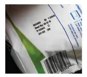
withstanding high temperatures are also available. Laser coders do not use consumables and work by removing a layer of substrate to create a code or mark.
