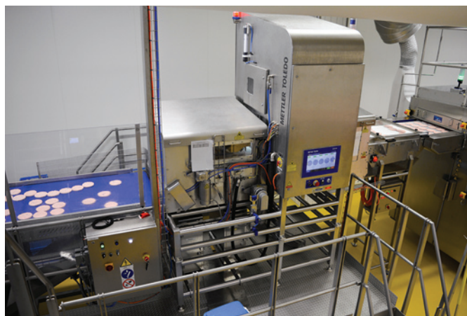
Bell Food Group is producing perfect burger patties using a new X39 x-ray inspection solution from Mettler-Toledo that checks for contaminants and defects.
