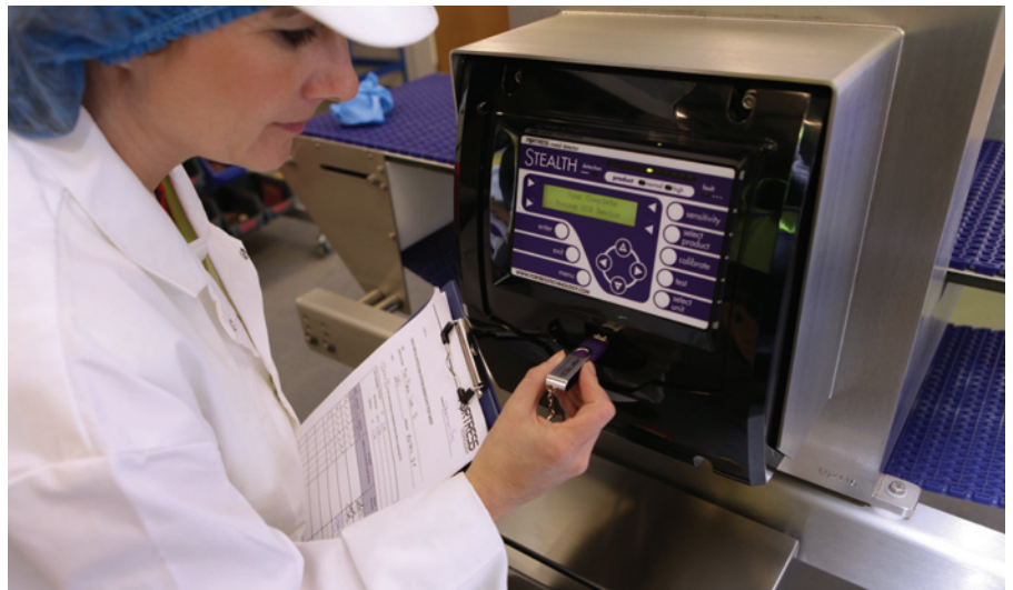
For full traceability, data can be automatically logged into many metal detection systems, which can be quickly recalled if needed.
