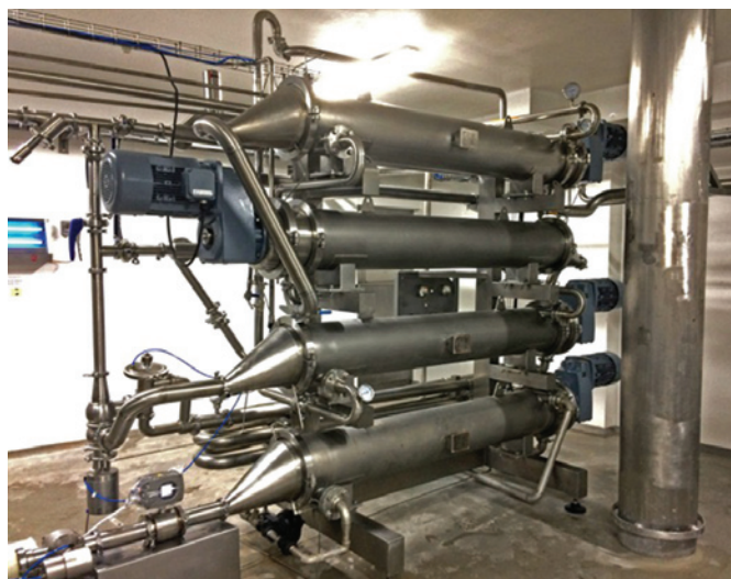
The HRS R Series can be run in reverse at the end of a batch to reclaim valuable products, effectively emptying the heat exchanger without damaging or affecting quality.
