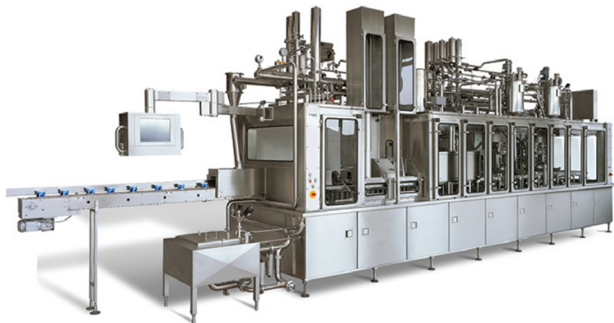
Carousel filling machine for pre-made bottles and cups, which is primarily used in the dairy industry.
