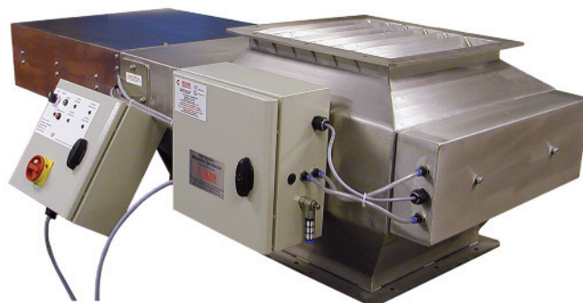
Eclipse Magnetics' Auto-Shuttle magnetic separator.
