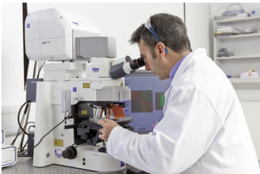
Using the confocal laser scanning microscope to look at foreign bodies.
