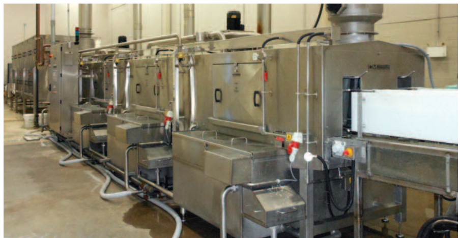
Papa John’s Dallas, Texas, commissary installed an automated two lane, four tank washing system to clean and sanitise its dough trays at the rate of 2,000 per hour. The photograph above shows a view of the infeed of the tunnel washer.
