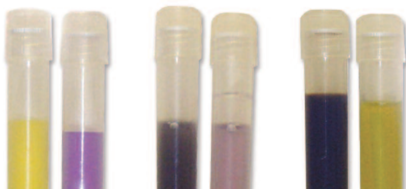
Path-Chek Hygiene Pathogen detection broth. Positive reactions are on the left and negative are on the right.
