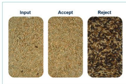
**An optical sorter is capable of identifying the dark ergot and separating it efficiently from the grain.**
