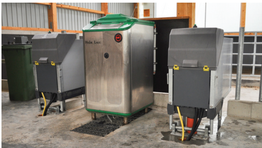
Automatic calf feeder with two Hygiene Stations.
